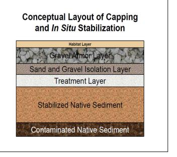
o clean sand will be placed on top of the "armor" layer to fill in the voids between the stones and to establish sufficient depth in order to restore the canal bottom as a habitat
