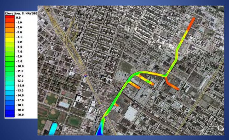
Bathymetric survey data provided by the U.S. Army Corps of Engineers, Engineer Research and Development Center
