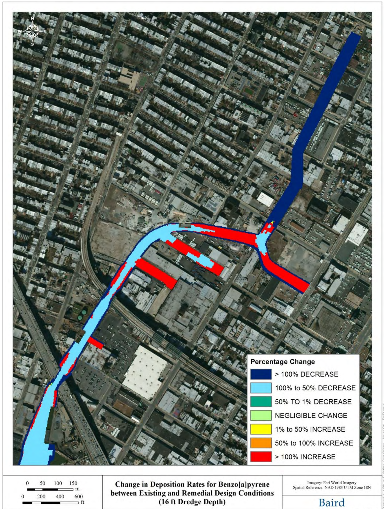
Figure 11. Change in benz[a]pyrene deposition rates resulting from dredging to -16 feet for a wet weather flow event
