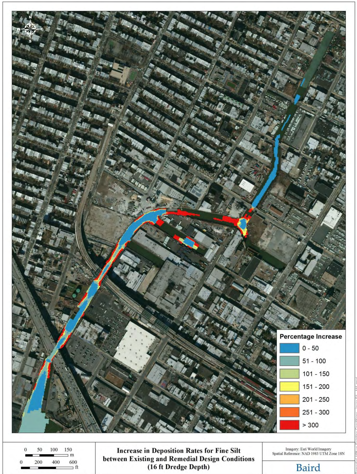
Figure 3. Increase in silt deposition rates in RTA 2 resulting from dredging to -16 feet
