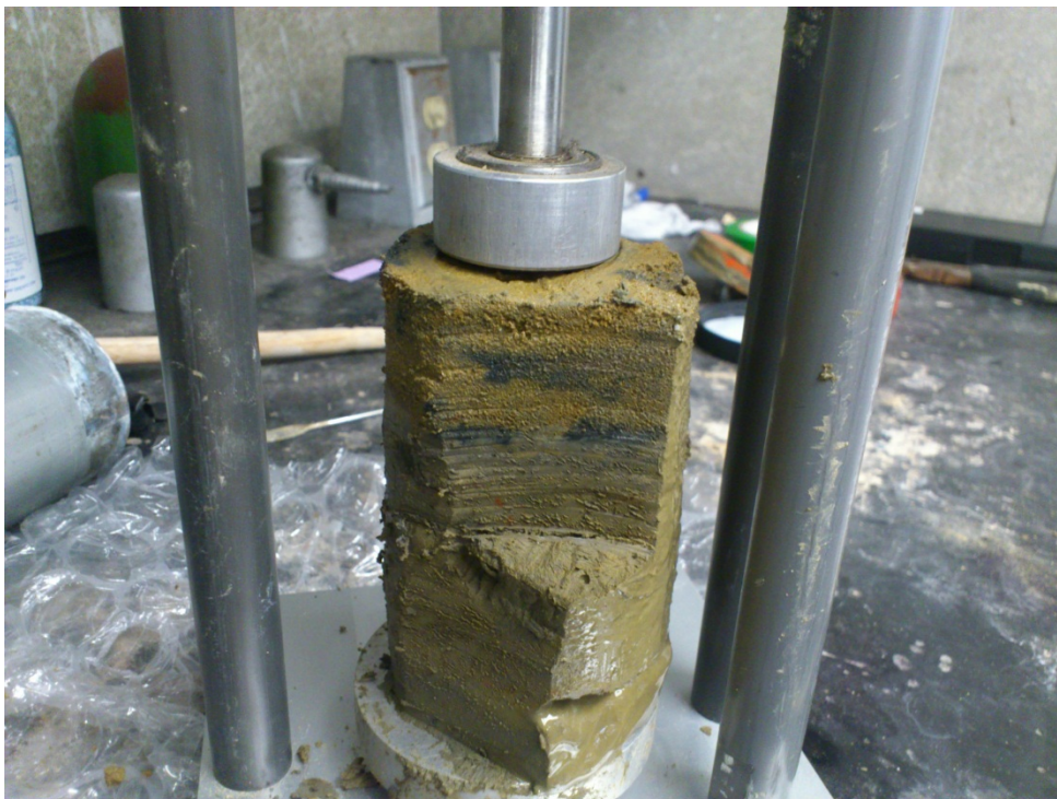
Figure 1: early stages of trimming on specimen GC-B-004(P1)
