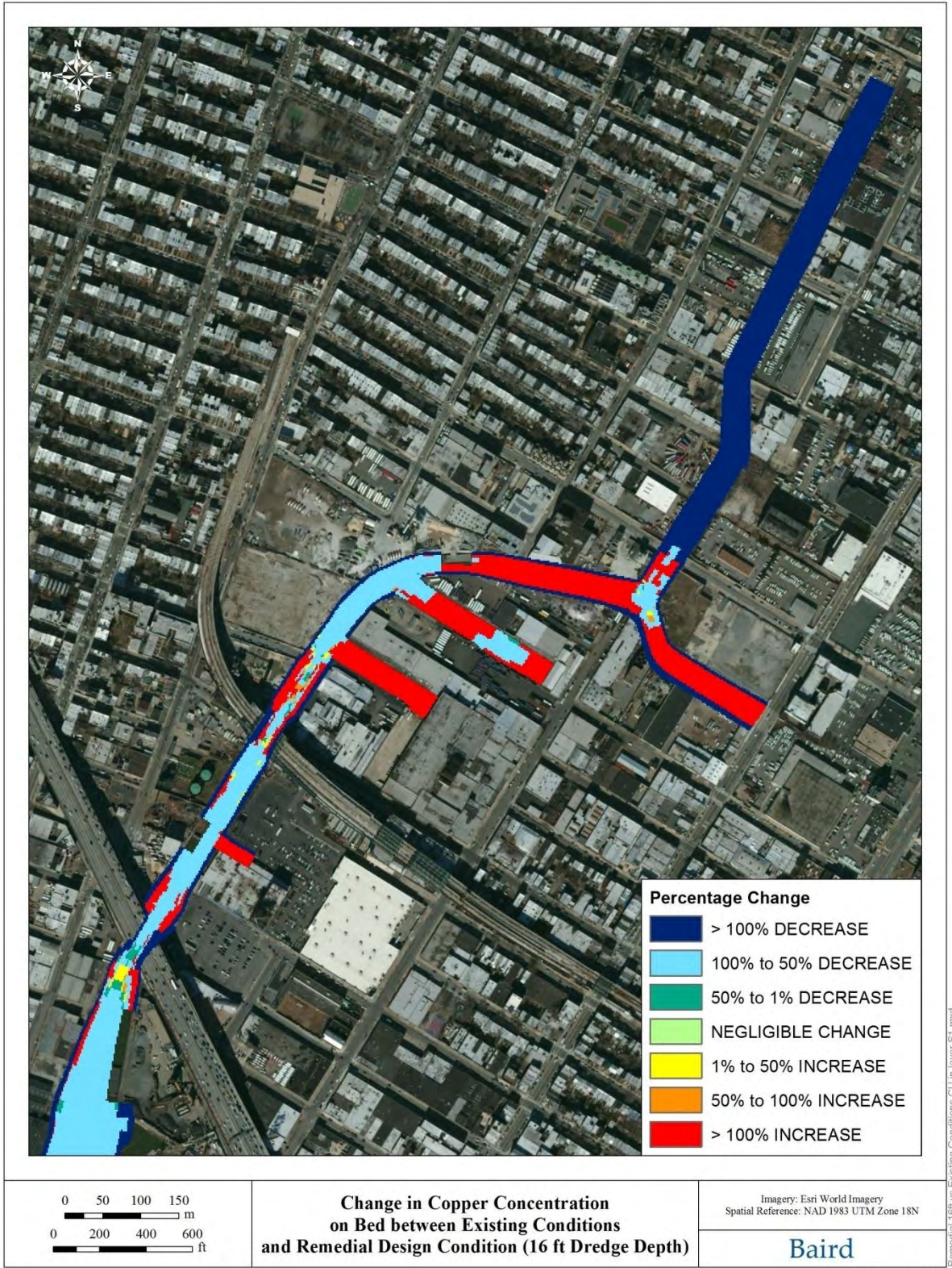
Figure 9. Change in copper deposition rates resulting from dredging to -16 feet for a wet weather flow event
