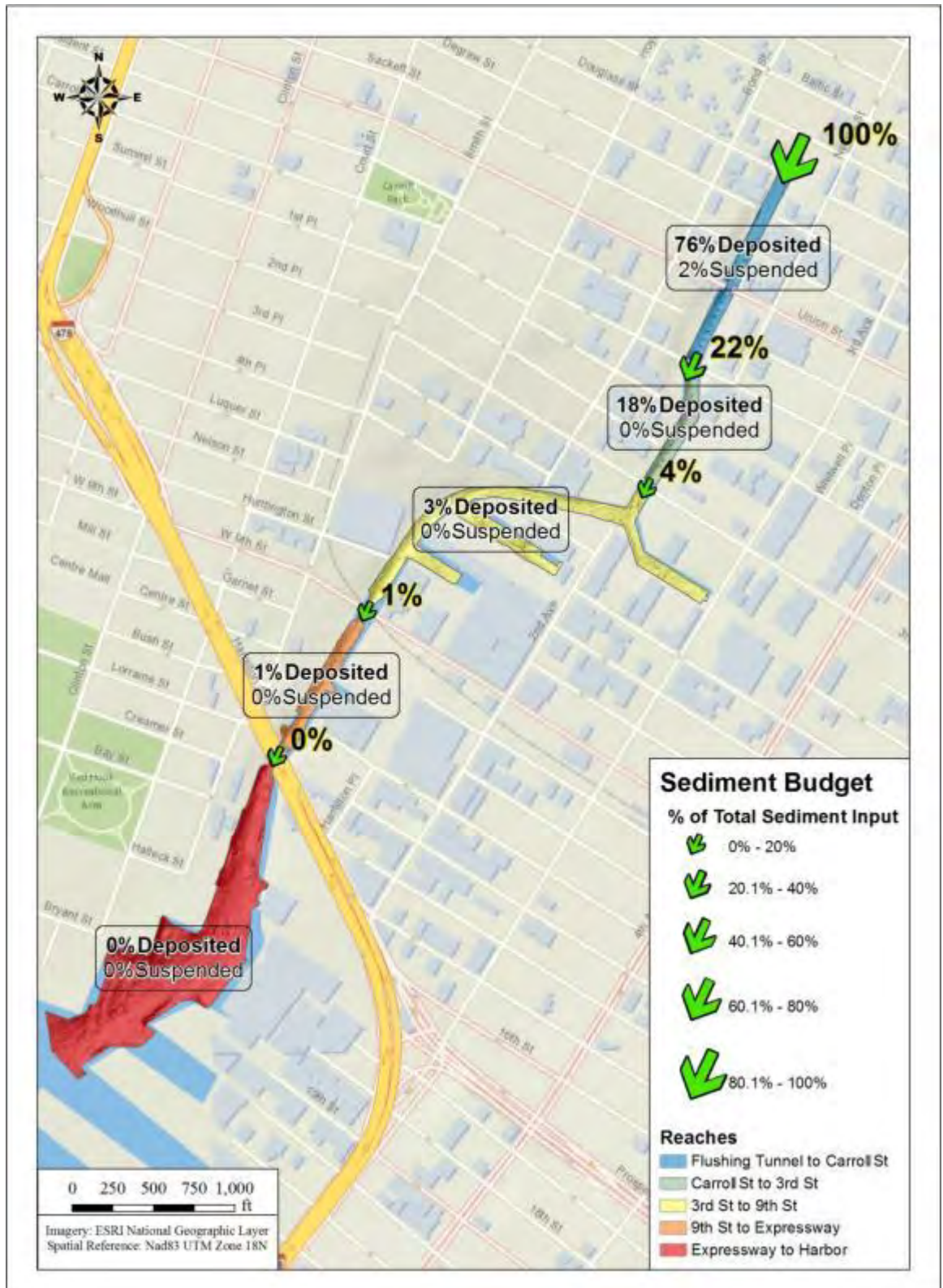
Figure 2. Fate of sediments introduced from CSO RH-034 under existing conditions, flushing tunnel inactive
