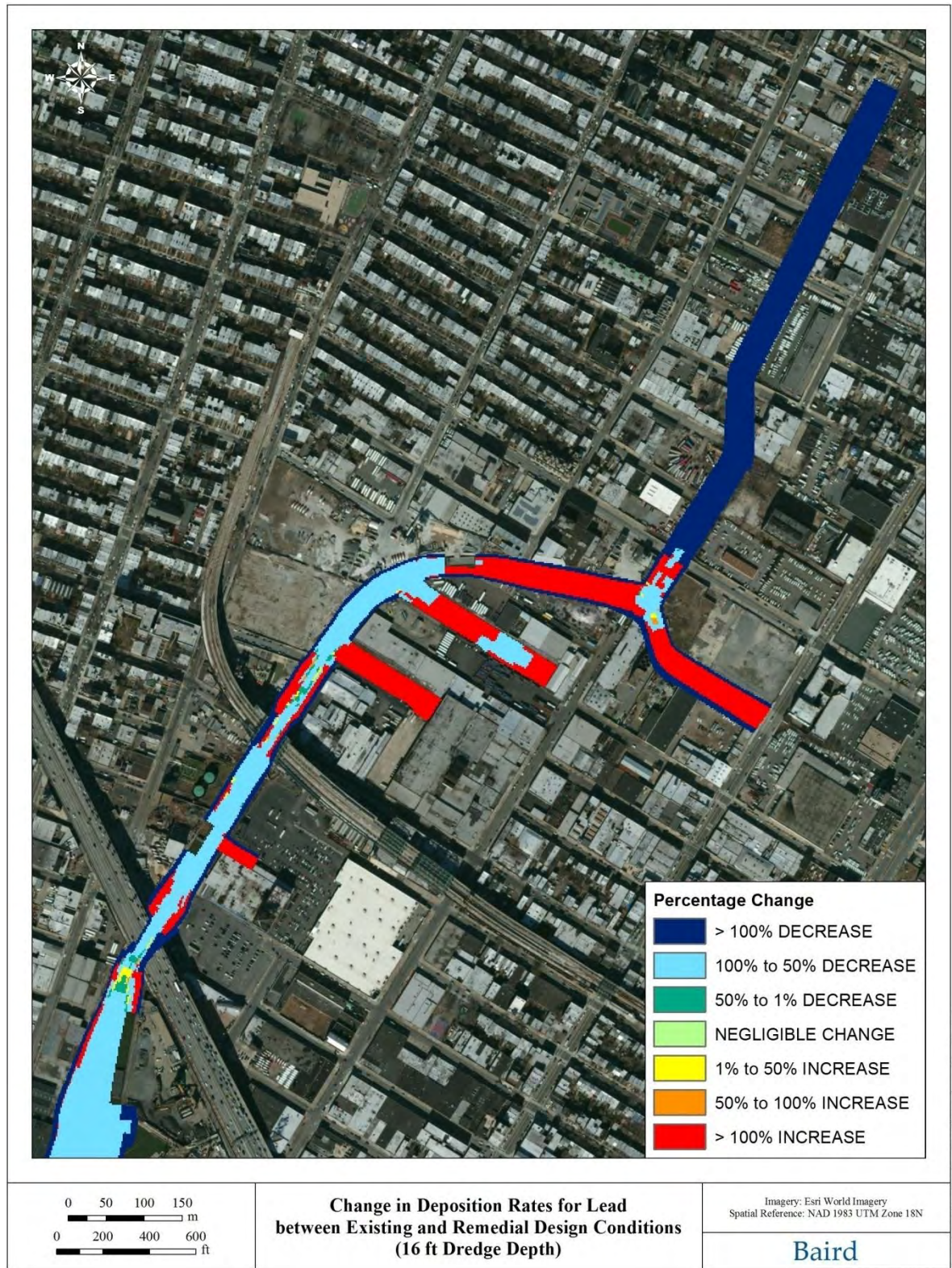
Figure 10. Change in lead deposition rates resulting from dredging to -16 feet for a wet weather flow event
