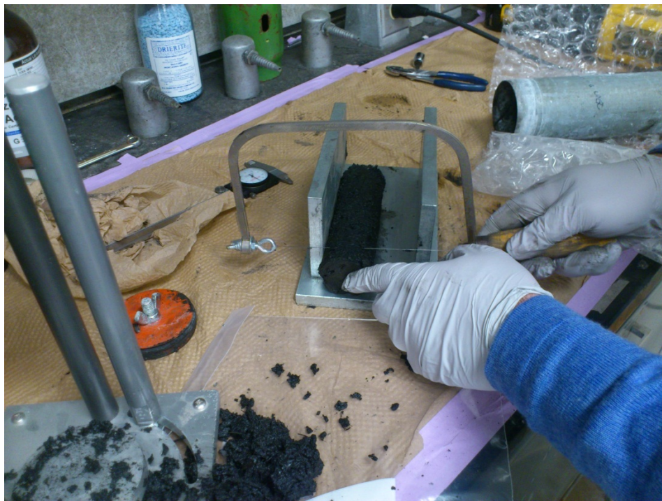
Figure 3: trimming top and bottom of specimen GC-B-002.
