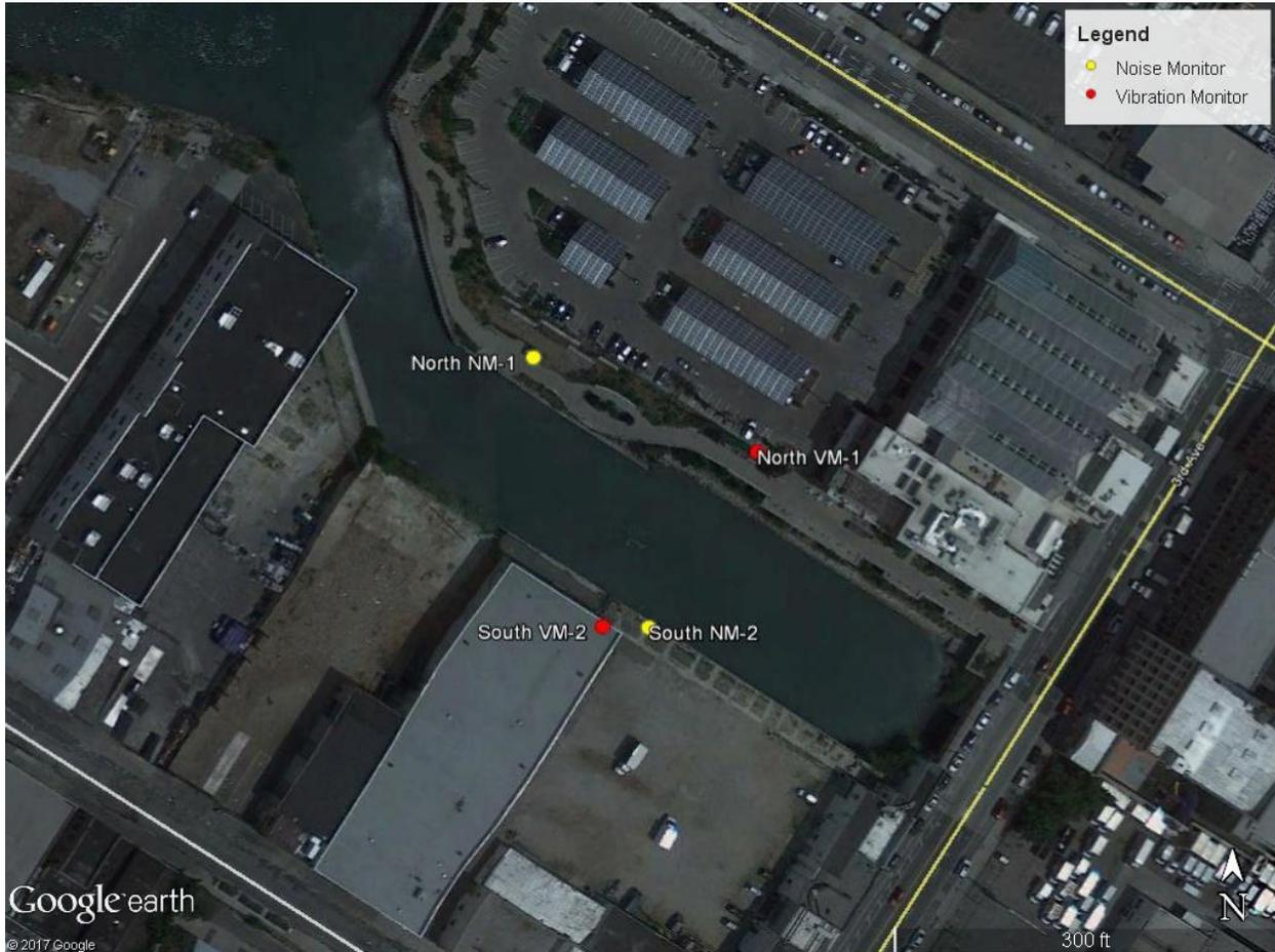
**Figure 1: Long-term Noise Monitoring Locations for Gowanus TB4 Dredging and Capping Pilot Study**
