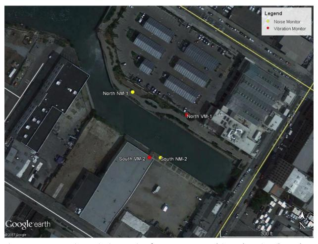
Figure 1: Long-term Noise Monitoring Locations for Gowanus TB4 Dredging and Capping Pilot Study
