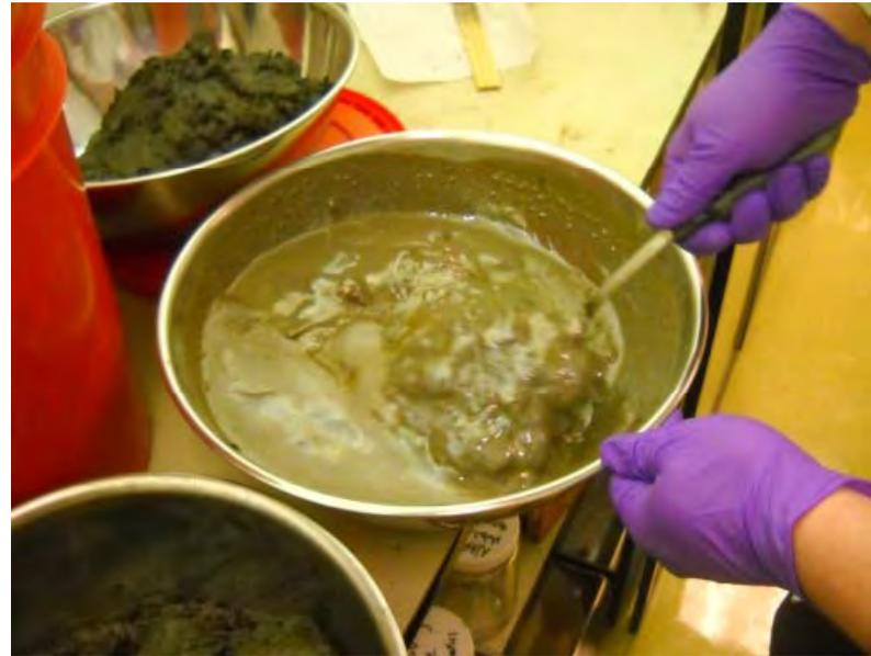
Cement agents and adsorbents mixed into a slurry
