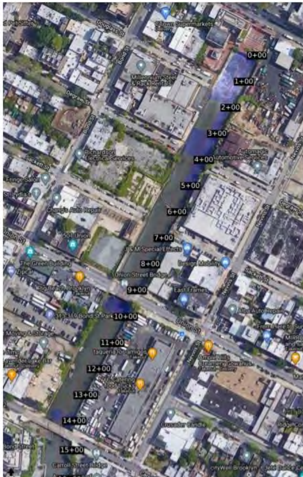
Figure 1 – Approximate area dredged on March 5, March 8 to March 12 and March 15, 2021. March 16 and March 17, 2021, sediment was raked between the 3 rd Street Bridge and Carroll Street Bridge in preparation for ISS activities with a negligible amount of debris removed. March 19, 2021, material was dredged in front of the flushing tunnel as part of a cofferdam exploratory investigation.
