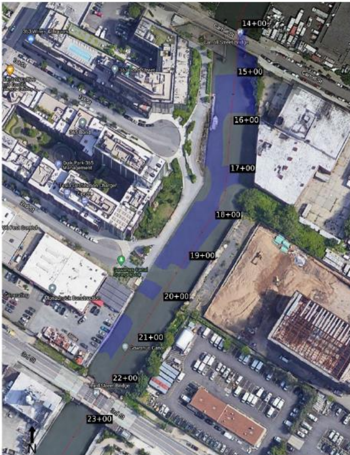
Figure 1 - Approximate area dredge between December 07, 2020 and December 11, 2020. Blue shading represents the approximate dredge areas. Figure provided by the Trust.
