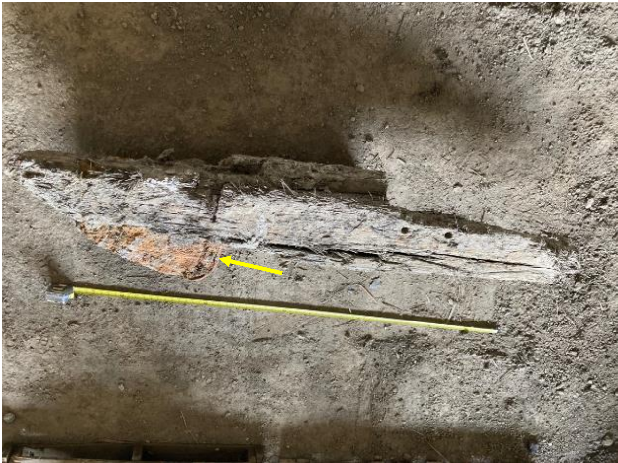
Photograph 21– Wooden timber with metal spikes (arrow).
