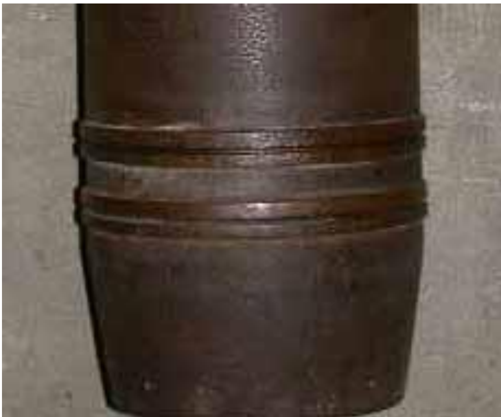
Photograph 29 - Example of two driving bands on an artillery shell. Source from Cartridgecollectores.org
