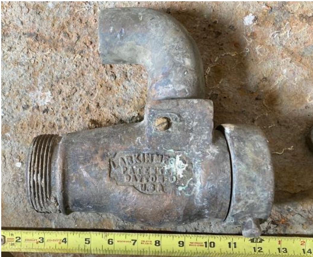
Photograph 2 – Brass component of a fire suppressant apparatus manufactured by the Larkin
