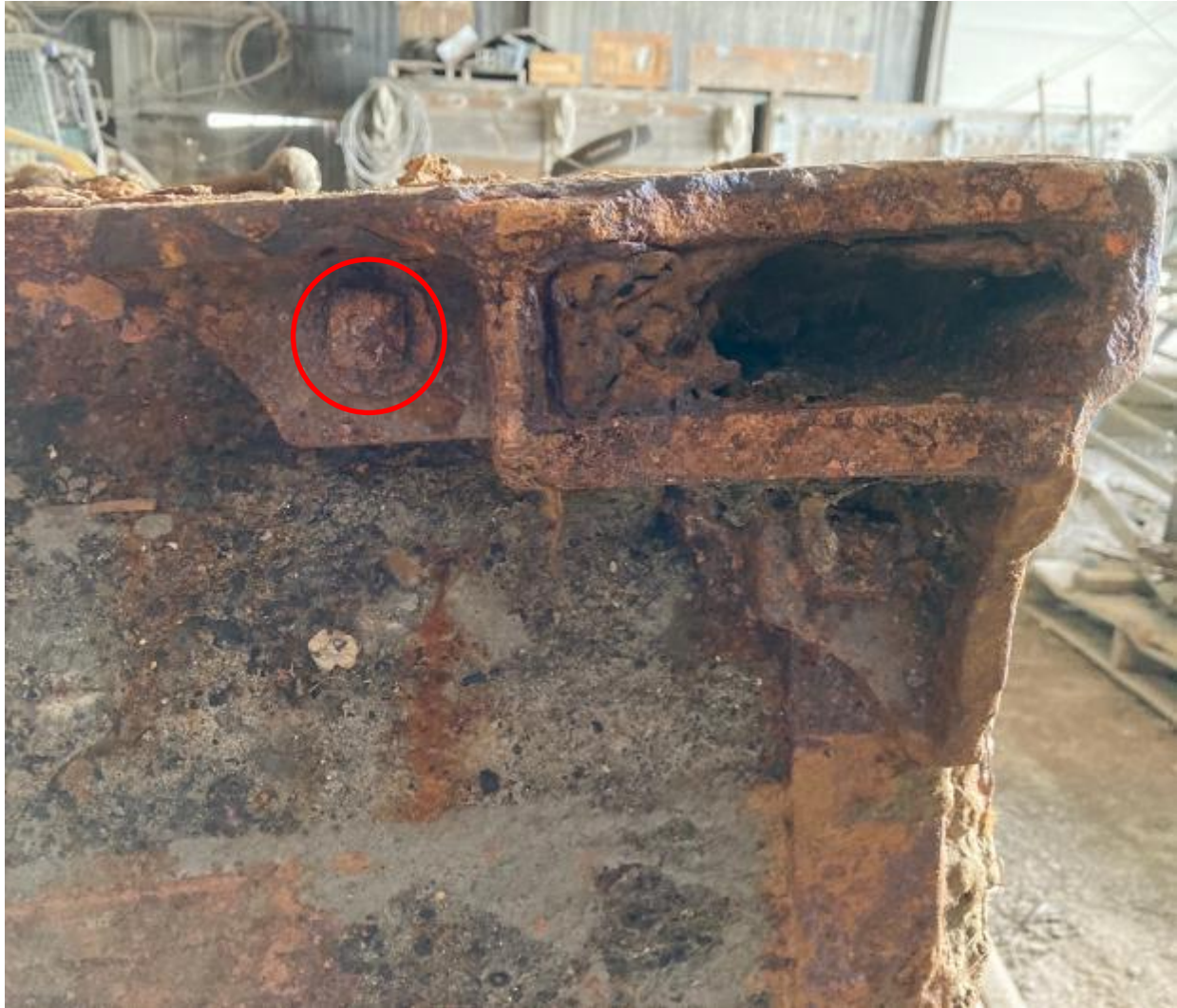
Photograph 15 – View of the square bolt attaching the foot of the safe (circle).
