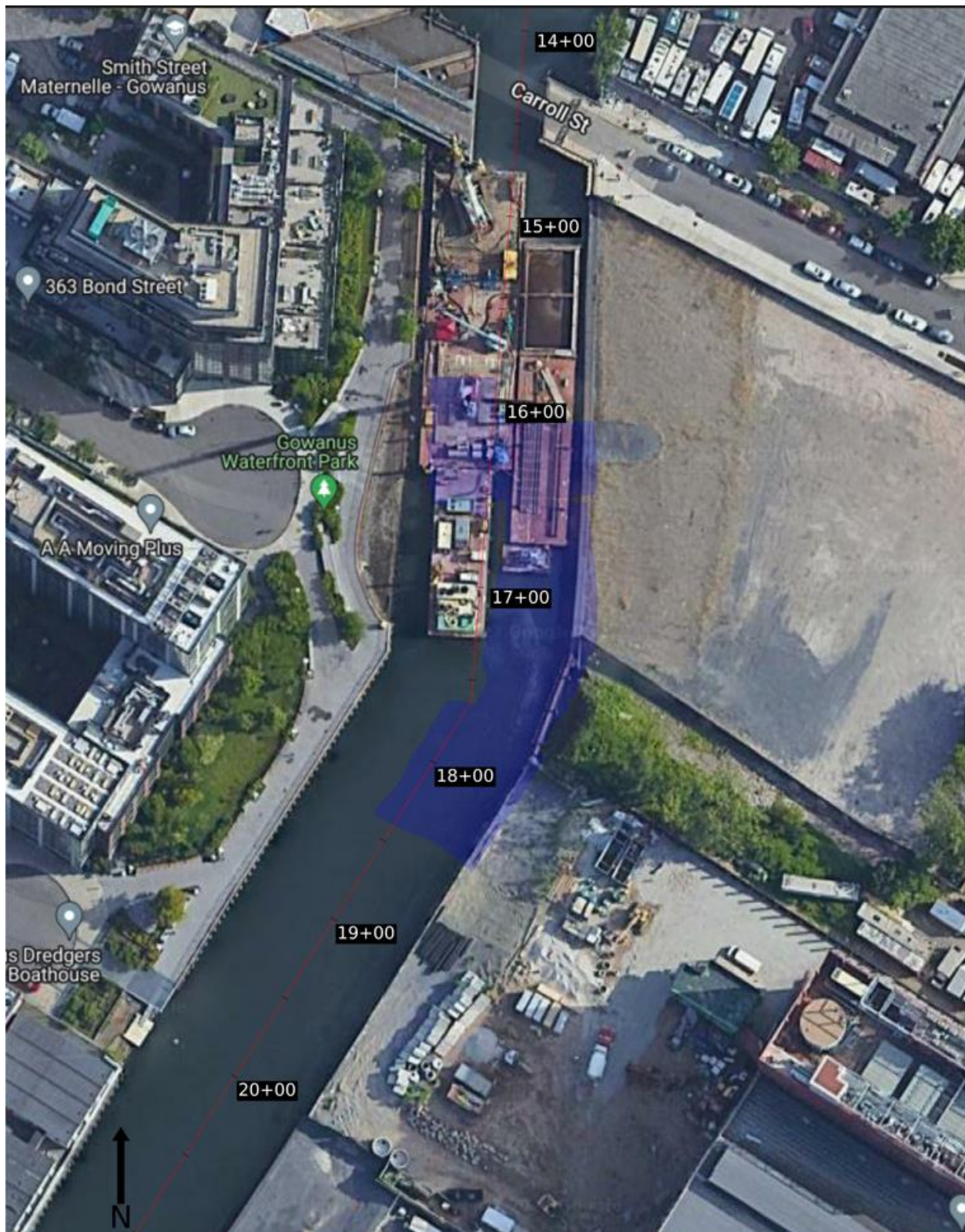
Figure 1 - Approximate areas of Phase III material dredged north of 3 RD Street Bridge between September 1 and September 9, 2022.
