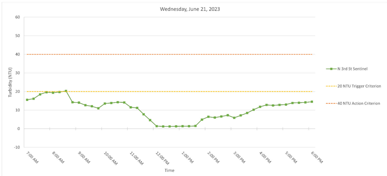
Figure 4. Hourly rolling average turbidity readings on Wednesday, June 21, 2023, from 7 AM to 6 PM.
