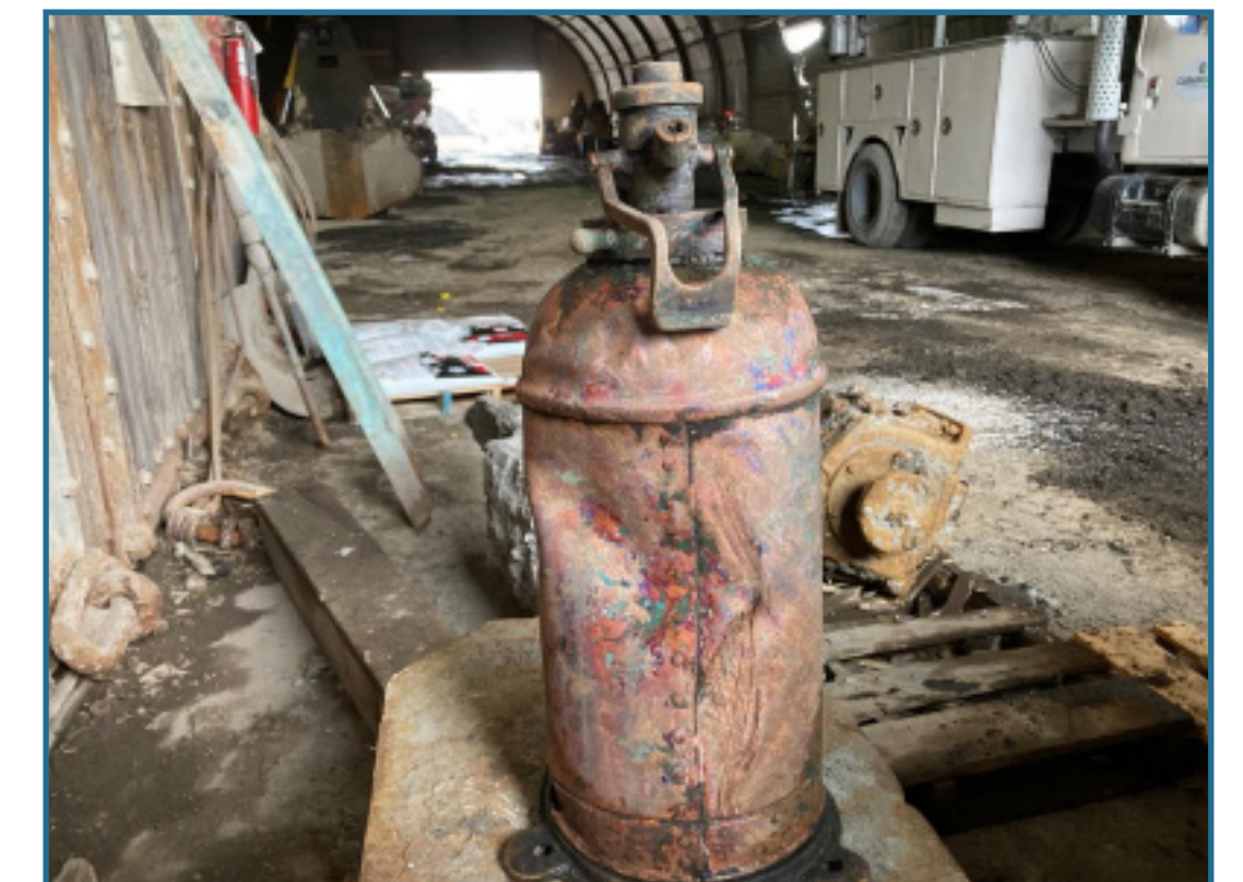
Copper fire extinguisher with rivets and nozzle, side view.
