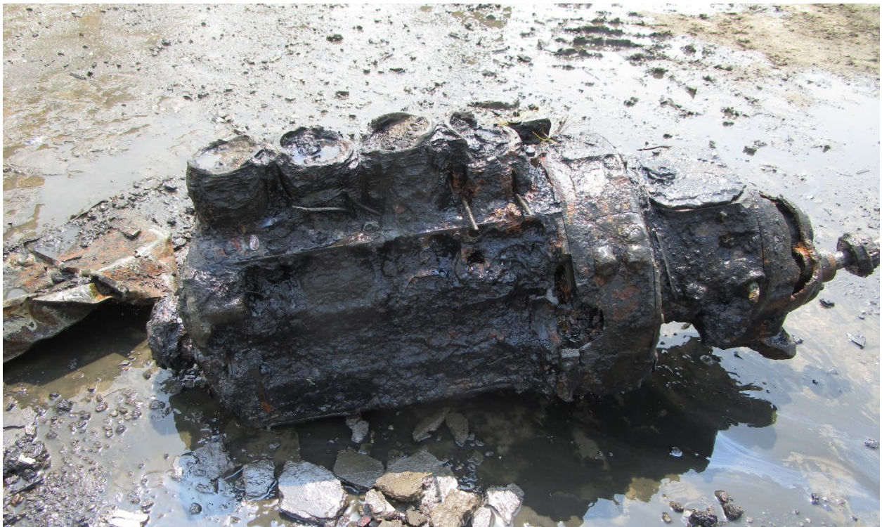
Photograph 3. Four-Cylinder diesel engine, incomplete (Chronicle Heritage, July 29, 2024).
