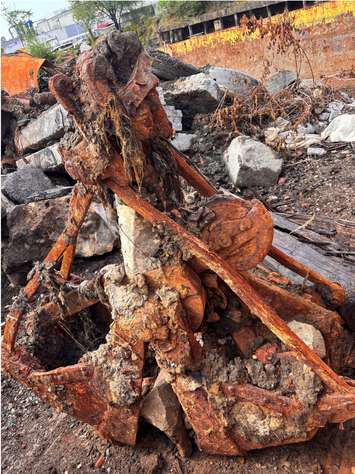
Photograph 4. Side and posterior view of bucket after thorough cleaning. Note the pulleys are entirely metal (Ben Romagnoli, July 1, 2025).
